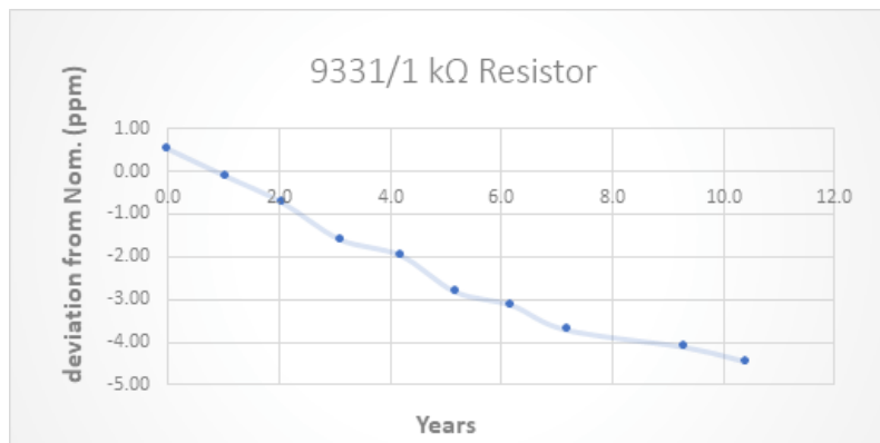
Figure 2. Drift of MI Resistor Over a 10 Year Period
