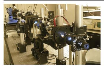
The Cryogenic Radiometer that is the CMI national standard of total radiation power.
