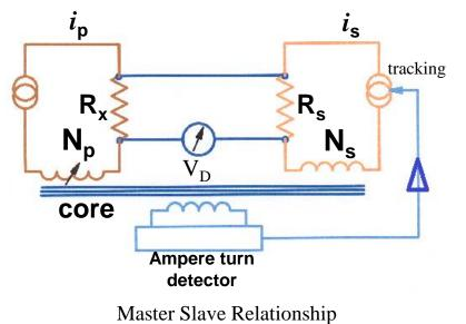
• The tracking circuit and N<sub>P</sub> are used to create and ampere turns balance in the comparator
