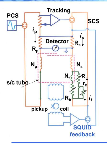
Cryogenic Current Comparator Bridge Ampere Turn Device & at balance  $i_p \times N_p = (i_s \times N_s) + (i_t \times N_t)$  $R_p \times i_p = R_s \times (i_s + i_t)$
