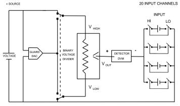
13 Bit Binary Voltage Divider 10V/2<sup>13</sup> = 1.2 mV DMM only sees voltages below 1.2mV
