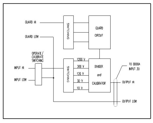
FIGURE 1 ... 8001 A SYSTEM SCHEMATIC
