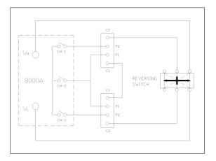
**RATIO VERIFICATION:** Where external resistors are used to verify the ratios of the 8000. If you don't have a JJ
