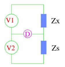
Usually, we use a bridge to scale from a known impedance to an unknown impedance.
