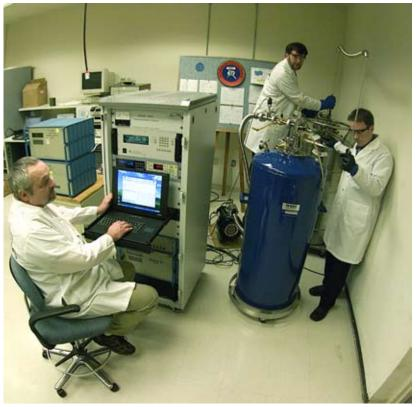
Installation of the Measurements International Quantized Hall Resistance Standard system at the Navy Primary Standards Laboratory, San Diego.
