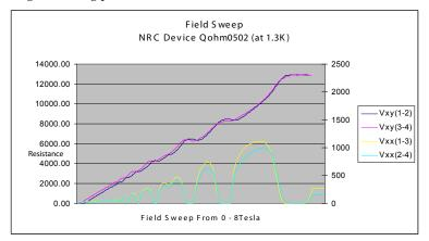
Figure 2. Sweep Check of QHR Device Q $\Omega$ 0502 (at 77uA) @ 1.3Kelvin. These field sweeps are representative of the data sets from a correctly cooled twodimensional electron gas (2-Deg).
