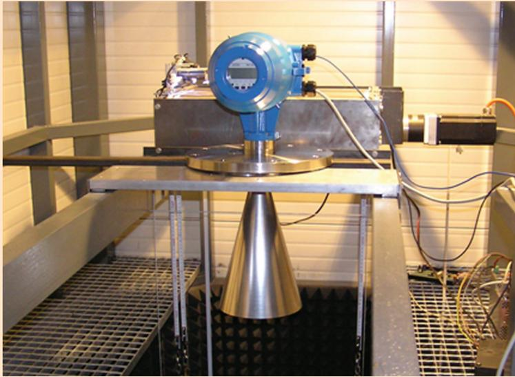
Radar level gauge being calibrated in the Laboratory of Flow and Heat.
